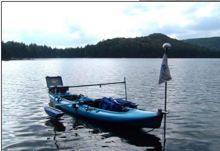
DT-X mounted on a kayak for use at a remote location. Courtesy of Darrin Freshwater Institute, Rensselaer Polytechnic Institute.
