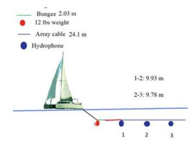
**Figure 1:** The hydrophone array trailing behind the *Gato Verde*. Photo courtesy of Dominique Walk As you can see the distance of the whole cable is 24.1 meters and the distance from hydrophone 1 to hydrophone 2 and hydrophone 2 to hydrophone 3 is 9.93 and 9.78 meters respectively. Also, a weight will be deployed with the array to keep it below the surface. The recordings will be made at 44.1 kHz, 16 bit sampling rate.
