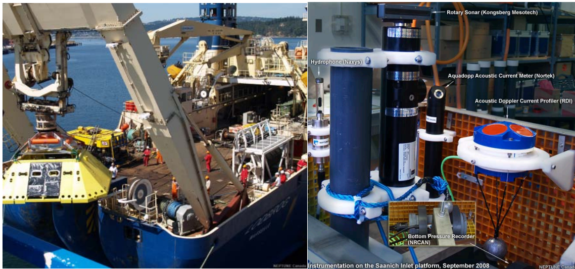
NEPTUNE instrument node heading to sea (left) and one location's instrumentation (right)
