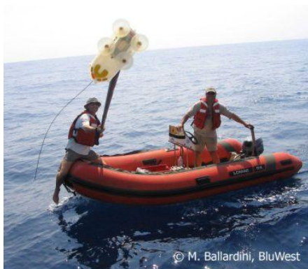
D-tag on pole, ready to be attached to a whale (or the photographer)
