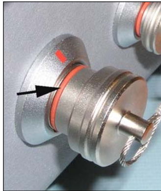
Connector protective cap – not properly inserted in connector.
