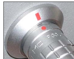
Connector halves properly lined up.
