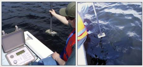
The VH110 hydrophone is used with a VR100 receiver to track small and medium sized tags.
