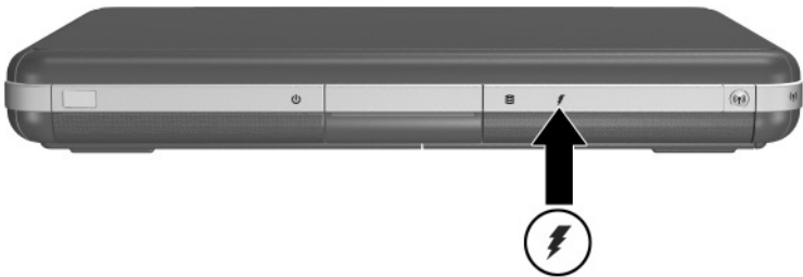
Identifying the battery light
