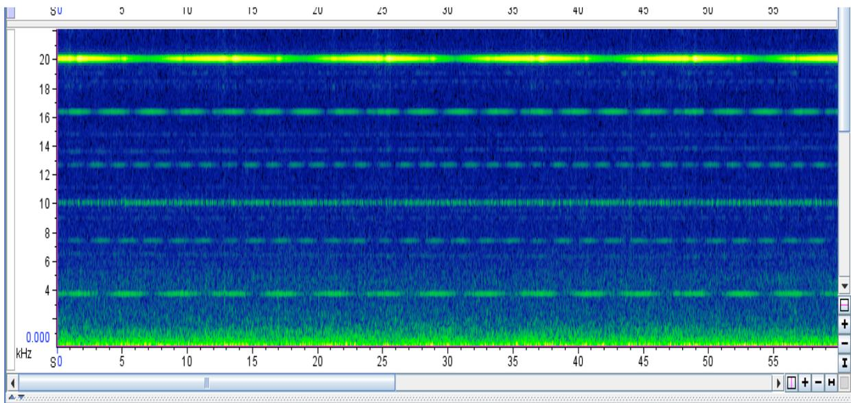
**Figure 3.** An example of electrical noise coming through the hydrophone recordings. Recordings like this were not used in the statistical sampling.
