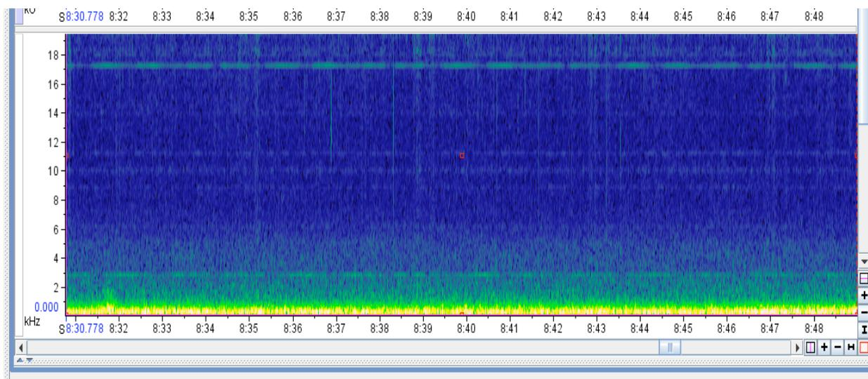
**Figure 4.** An example of light electrical noise coming through the hydrophone recordings. Recordings like this were acceptable for use in the statistical sampling.
