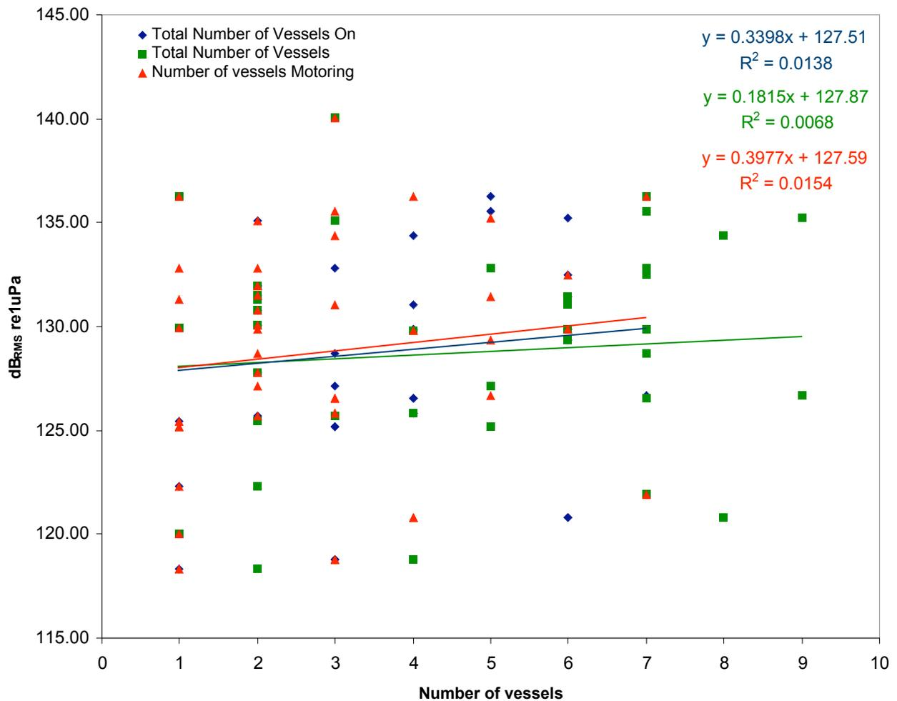
**Figure 1.** Relationships of vessel noise and the different category states of vessels.
